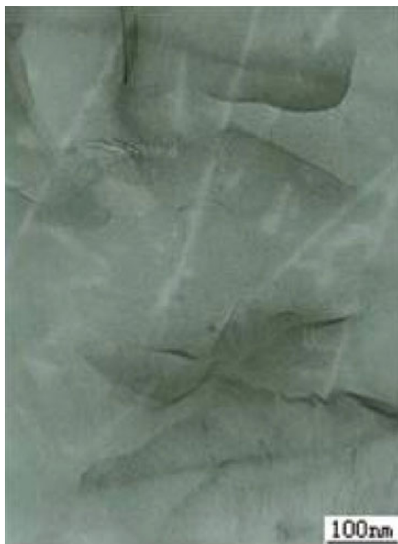
Figure 2 TEM micrographs of NGPE with 5 wt % OREC. [Color figure can be viewed in the online issue, which is available at www.interscience.wiley.com .]
